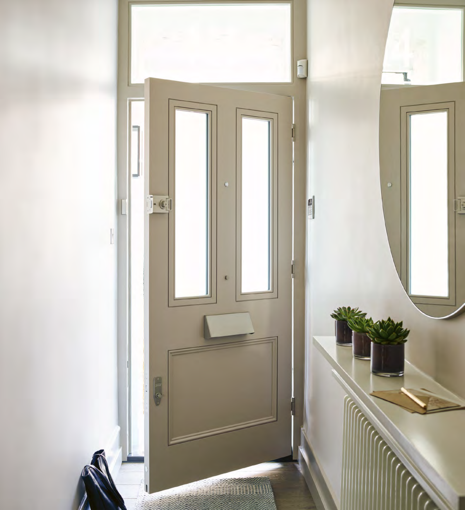
Banham High Security Door , frame & fanlight with toughened laminated glass, fitted with satin chrome locks operating from the same key, letterbox protector & doorview. Banham Alarm Keypad, flush door contact & passive infrared detector shown.
